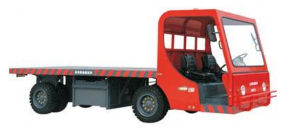
• Battery can be side-pulled out from the truck, improve working efficiency.
